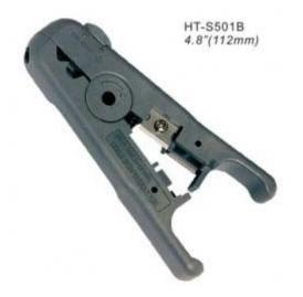
For wire (UTP/STP) or wire and multi conductor cable from 3.2 mm-9 mm max. Irregular out-shape insulation can be put the front "V" and "U" guide, rotate the tool 1-3 times by index finger for stripping the outer insulations easily also has adjustable knob for fitting different cable sizes.
